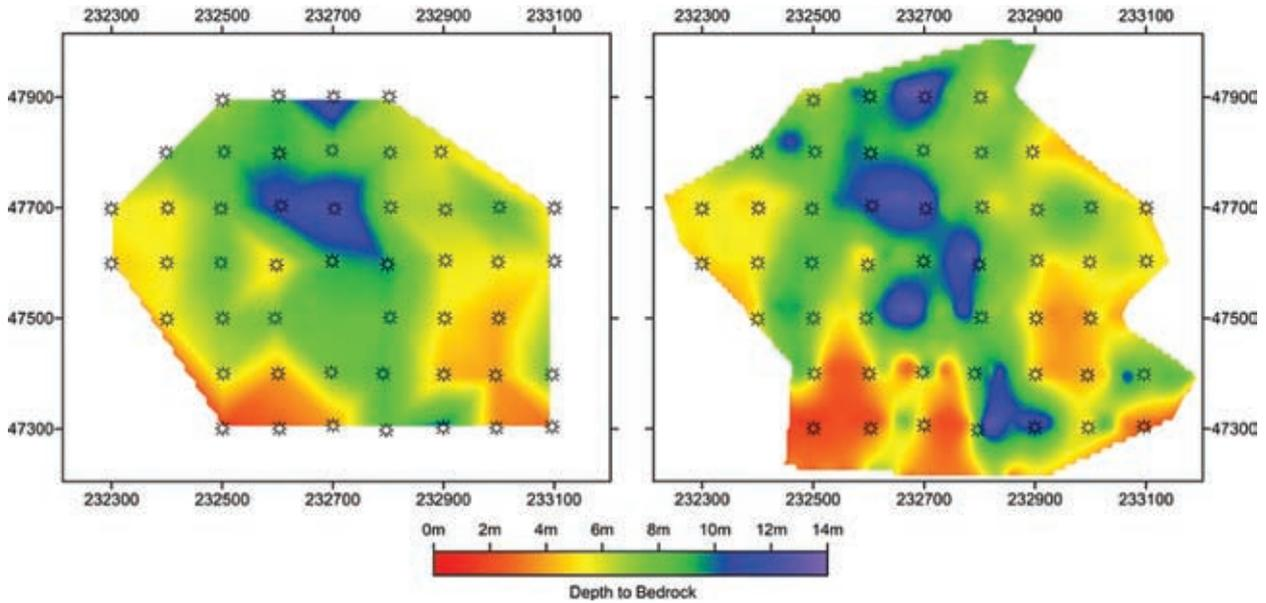
Figure 5 Comparison of isopach map of depth to bedrock beneath a lateritic weathering environment generated by drilling along (left) and by GPR (right). Note the GPR data correlates well with the drilling depths but provides significantly more detail between holes.
