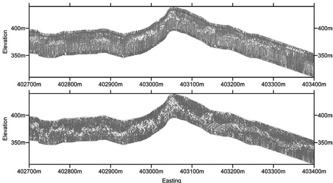
Figure 3 Comparison of saprolite horizon as imaged by commercial GPR (top) and real-time sampling GPR (bottom).
