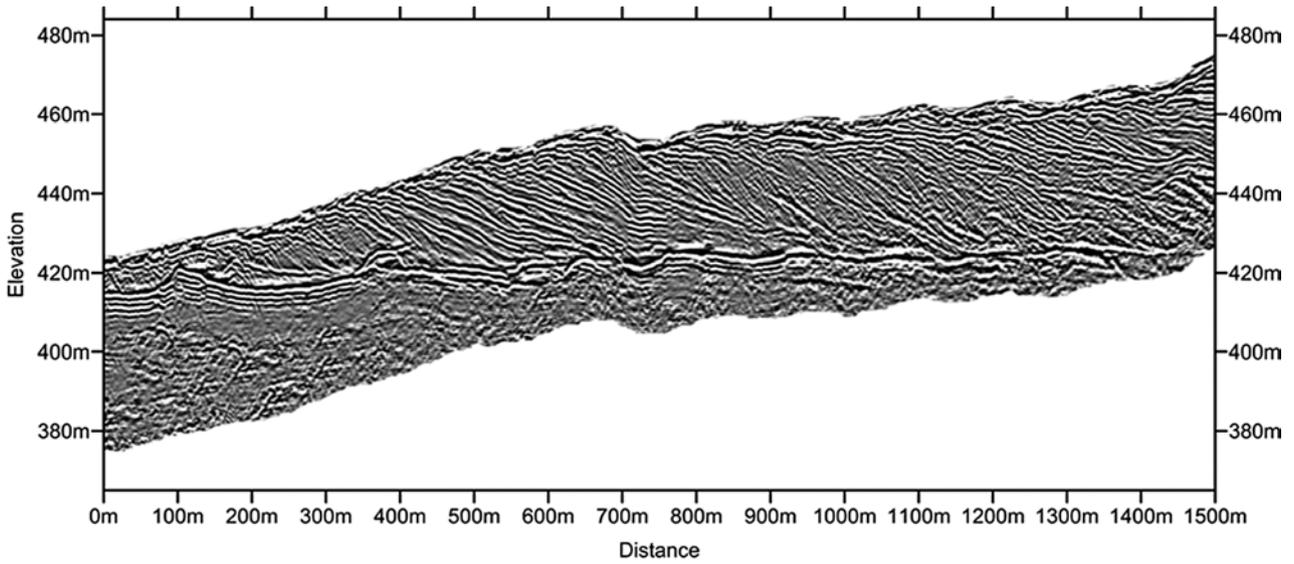
Figure 11 Modern GPR systems may be towed over sand dunes at high speed, producing high-resolution images of dune stratigraphic.
