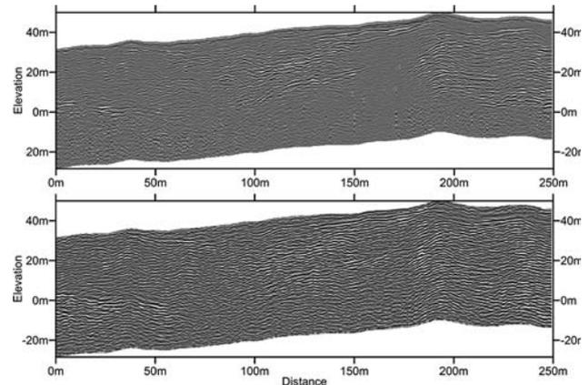
**Figure 10** Comparison of commercial GPR with 50 MHz antennas (top) to newly developed GPR (bottom) over silica-rich sand dunes.
