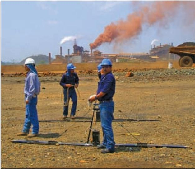
Figure 1 Commercial GPR system with 25 MHz antennas.
