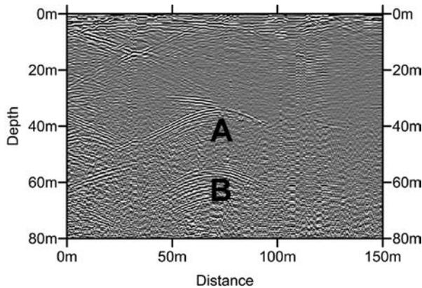
**Figure 9** Example of long-range imaging of voids in coal strata (A and B). Other layered reflections below 30 m are coal strata whereas those above 20 m are due to above-ground reflections.
