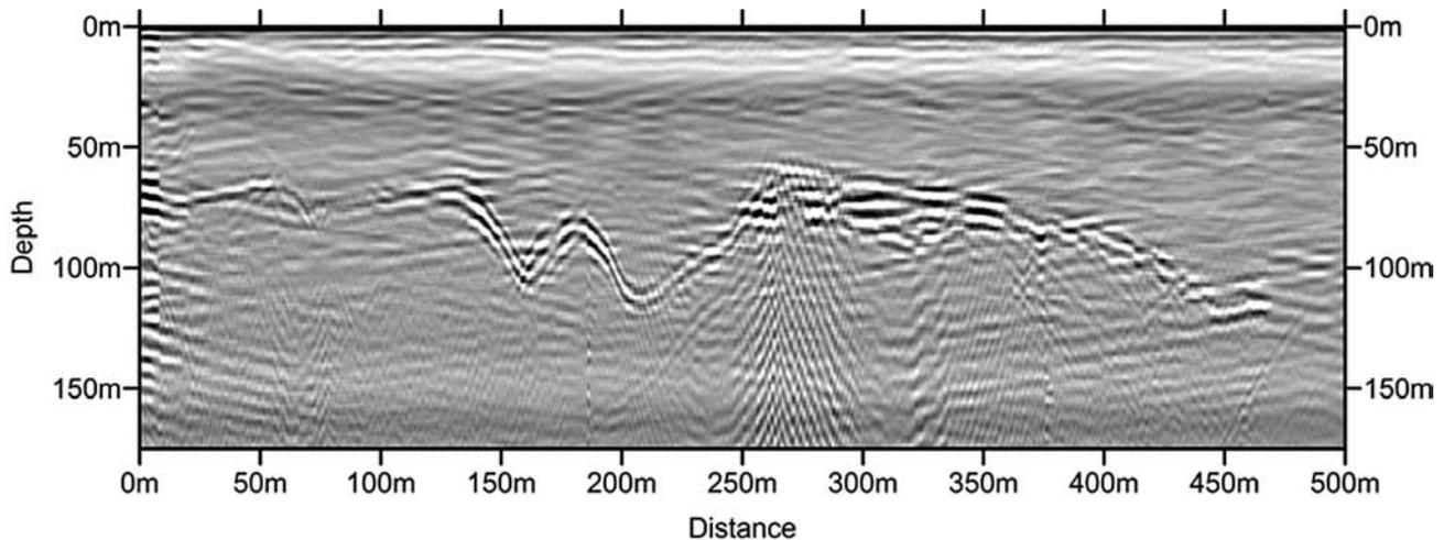
Figure 14 Image processing revealed the base of the waste dump to depths approaching 130 m.
