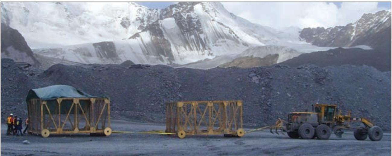
Figure 13 What are believed to be the largest mobile shielded GPR antennas built surveying a mine waste dump.
