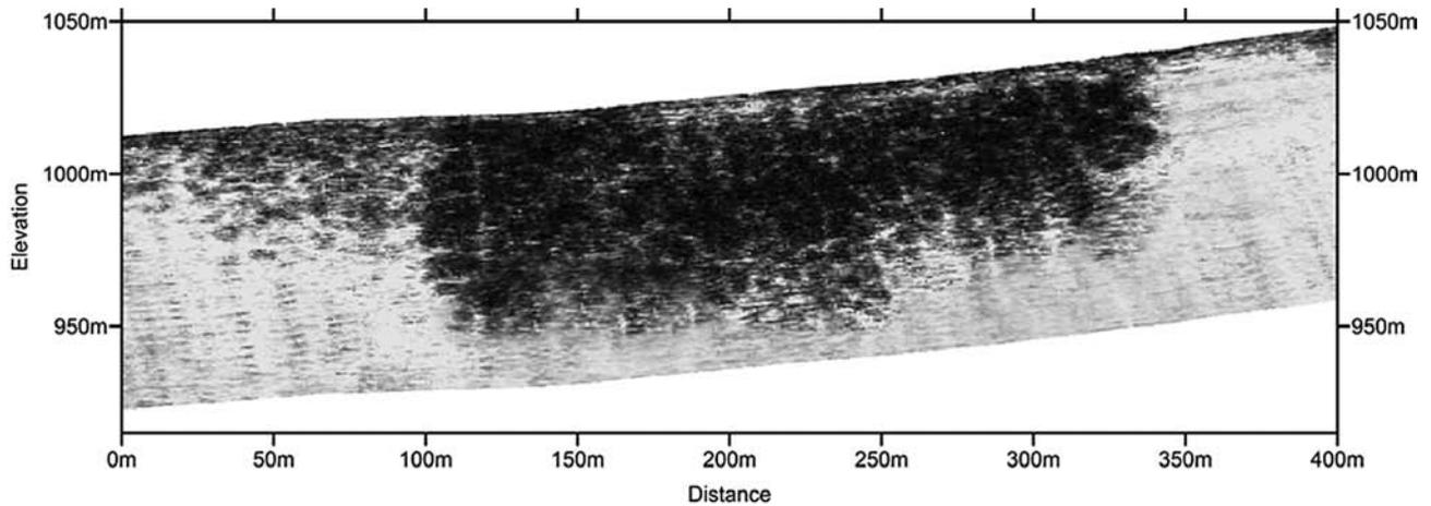
Figure 7 Profile showing the thickness of iron ore (dark region) generated with newly developed GPR.
