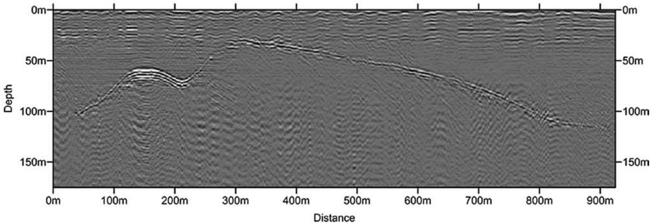
Figure 12 Example of data acquired with pulse-compression GPR showing base of sands to depths of over 100 m.
