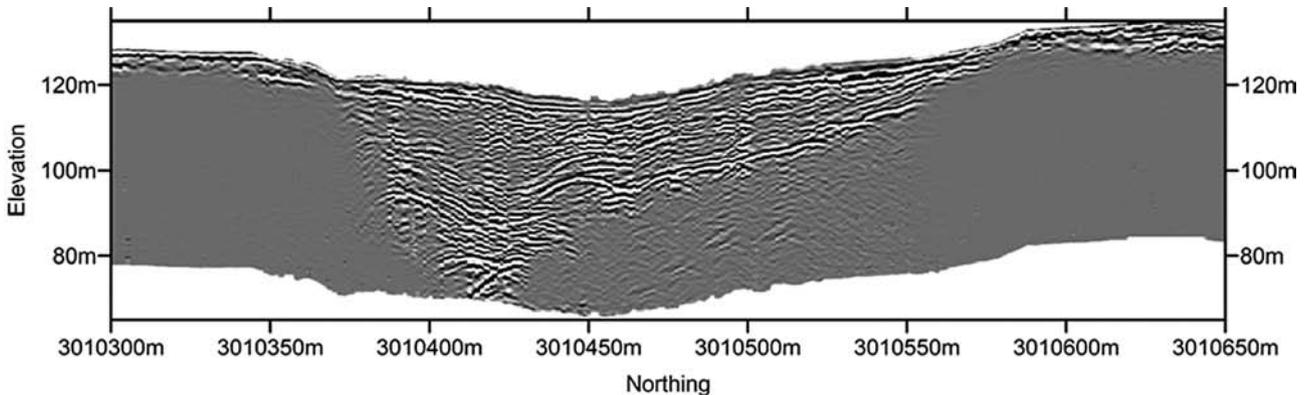
Figure 6 Data acquired over a paleochannel using a newly developed GPR system showing penetration to 40 m.
