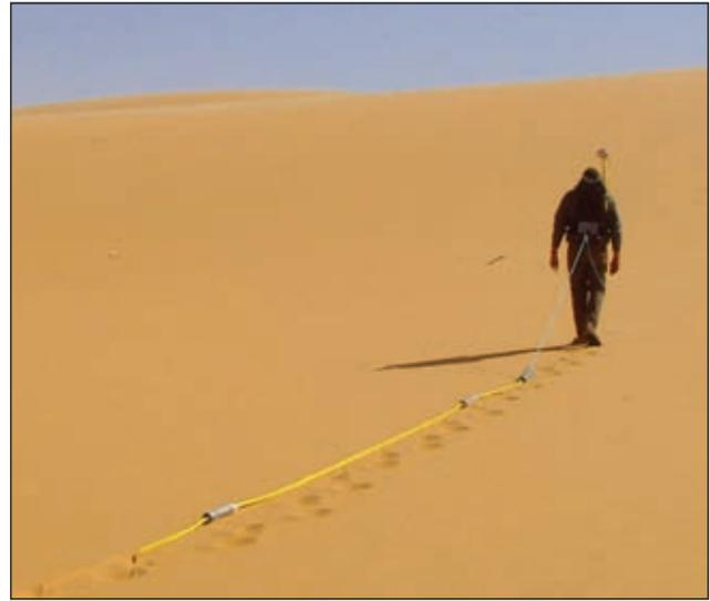
Figure 2 Newly developed wireless real-time sampling GPR system.
